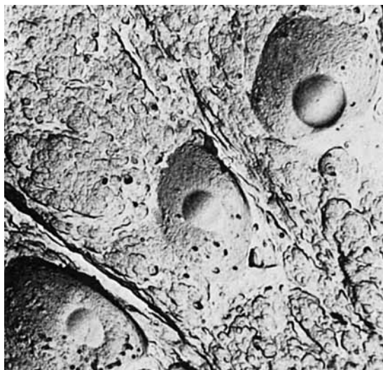
Fig. 2. Replica of a fracture surface of I generated under liquid nitrogen, corresponding to a string of voids such as was shown in Fig. 1. The round centers (voids) are surrounded by polymer which exhibits a smoother fracture morphology than the majority of the matrix. See text for explanation. Electron micrograph \times 8,640 .
